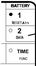
**DATA:** The **DATA** mode is used to recall key historical information about the battery (battery banks).
