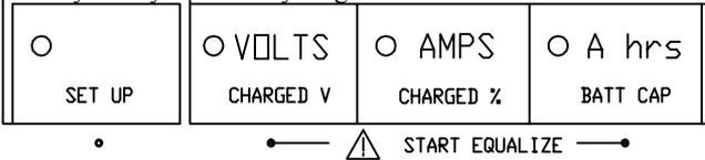
**CAUTION! Turn off voltage sensitive DC loads before equalizing battery!**
