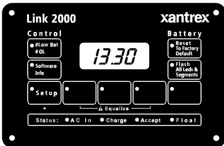
**# LOW BAT/ # OL:** The number of Inverter Low Battery shutdowns (since last reset) is displayed with a minus sign (negative number). The number of Inverter shutdowns (since last reset) from other causes are displayed with no sign (positive number). The display alternates at three-second intervals until the button is released.
