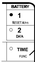
**FUNC:** The **FUNC** (Function) mode is used to set up special functions or features that are not commonly changed. They might be thought of as internal software switches that allow the selection of special functions, or values that, once set, are seldom changed.
