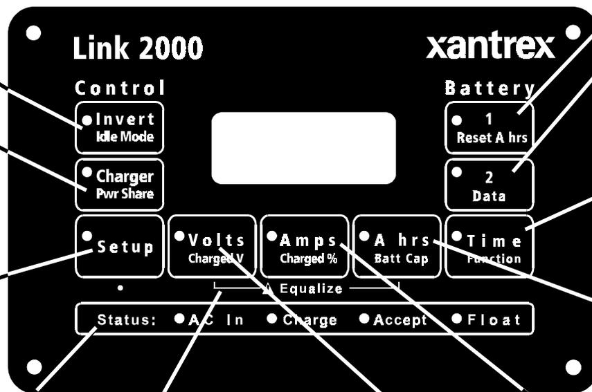
**START EQUALIZE** function of charger by pressing SET UP button for 5 seconds followed by simultaneously pressing the VOLTS and A hrs buttons until the "E" in the display goes out (3 sec.). Red CHARGE LED flashes when in equalize mode.
